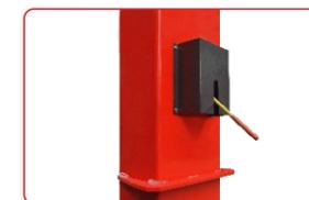
Single-point safety release makes it easier for operators to unlock both column locks from one column.
