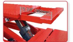
Extendable varying platform suitable for varying wheelbases
