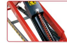
Mechanical lock and air-driven safety release.
