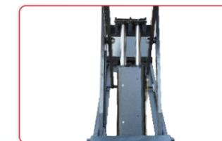
Dual hydraulic synchronization & hydraulic locking system;
