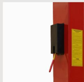
• Single Point safety release makes it easy for the operator to unlock both column locks from one column.
