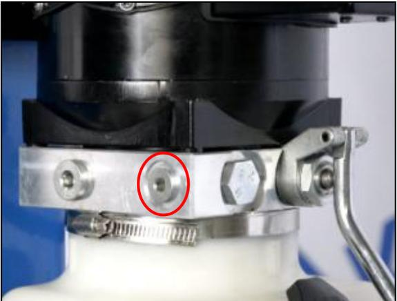
D. Install the iron plug from step A to the oil outlet port on the left side.
