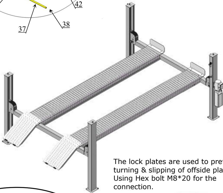
The lock plates are used to prevent the turning & slipping of offside platform, Using Hex bolt M8\*20 for the connection.
