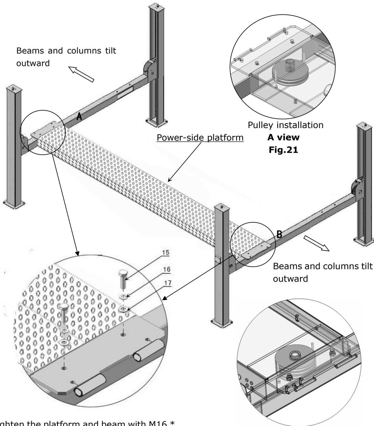
Tighten the platform and beam with M16 \*
