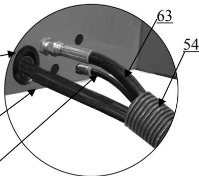
Cross beam limit switch cable and the oil return pipe all comes out through this hole
