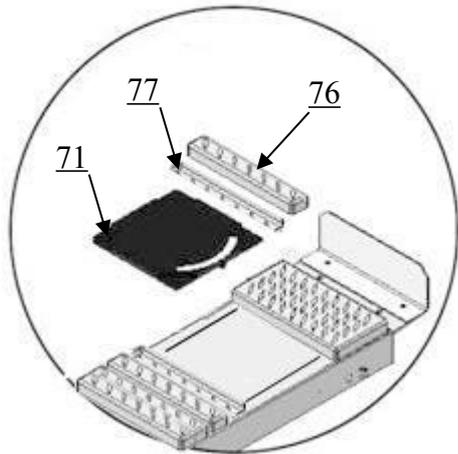
When installing the turntables, both sides are required a 35mm-high turntable block.
