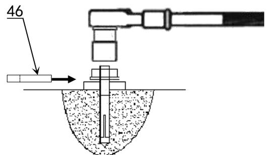
Using the ratchet spanner with socket to tighten the
