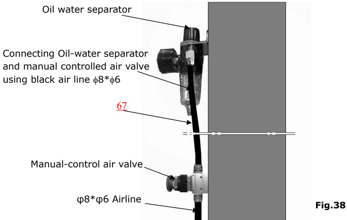
5. Connecting air inlet (Air supply pressure  $5 \text{ kg/cm}^2 - 8 \text{ kg/cm}^2$ ), adjusting the air pressure of Oil-water separator to 0.8 MPa **(See Fig.39)**
