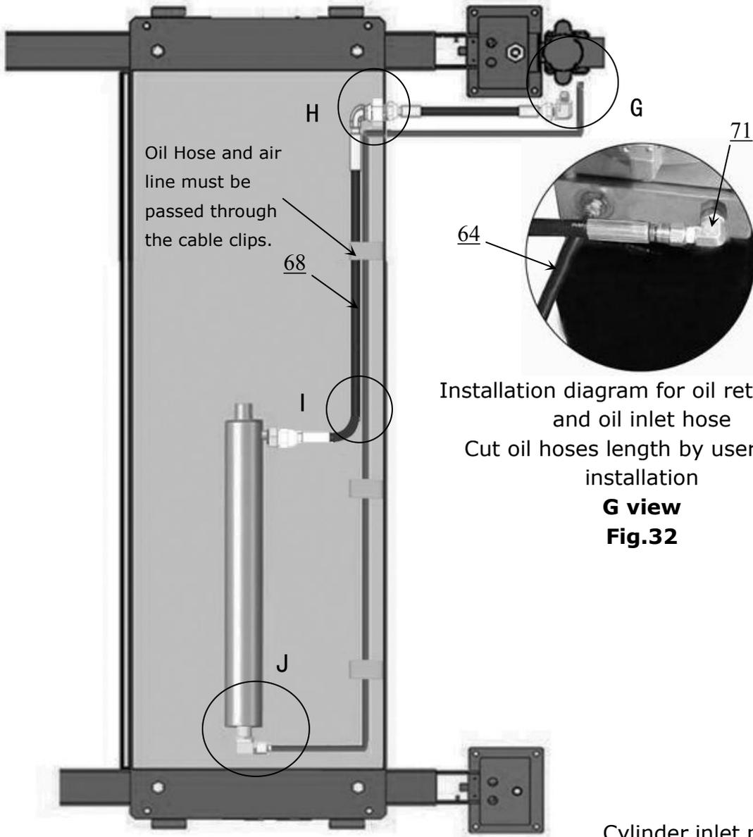
Installation diagram for oil return hose and oil inlet hose
