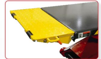
Adjustable ramps and extended platform for longer vehicles.
